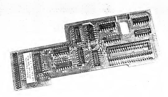
**THE SPRINTER™** by Holmes Engineering A keyboard installed speed-up module.
